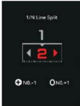
Once the 1/N value is set, press the measure key or pull the tape measure to confirm and start measuring. The total value will be displayed in the top left corner of the screen; the value of each interval will be shown in the top right corner. Move the device straight on the surface, and the indicator arrow will move accordingly. When a red arrow appears on the right and aligns with a green line, it indicates you've reached a division point.
