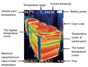
Temperature range: The range of temperature measurement (HT-19 automatically adjusts the temperature range, and the range icon is not displayed on the interface.)
