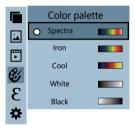
As shown in the figure, press "MENU" key to enter the main menu and select " (color palette) option and press " > " key to enter the color palette list. Press " ▲ " and " ▼ " keys in navigation to select the color palette. Then press "SELECT" key to select the color palette. Press " ◀ " to return. Press " MENU " key to exit from the menu.
