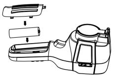
Take care to slide the battery cover into the correct position of the handle.
