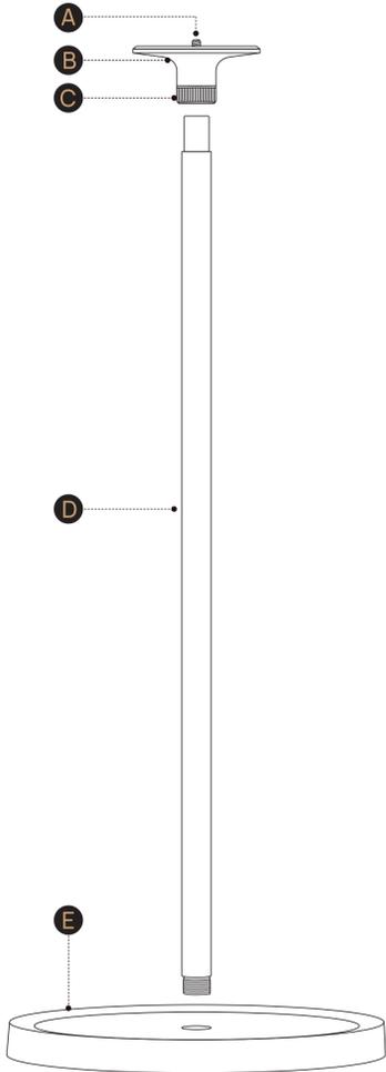
**1** Position the base in the appropriate location, align the threaded end of the support rod with the center of the base and tighten the rod clockwise.
