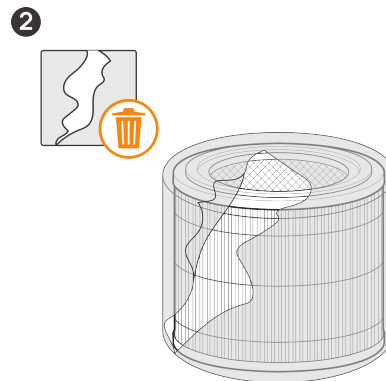
Step 3: Remove plastic packaging from the filter
