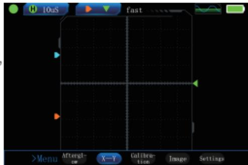
**X-Y:** You can enter X-Y display, at this time, measurement, cursor, calculation are all useless.
